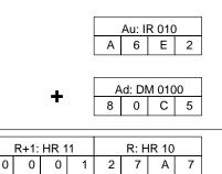
**Note** The UF and OF flags would also be turned ON during this addition, but they can be ignored since they are relevant only in the addition of signed binary data.
